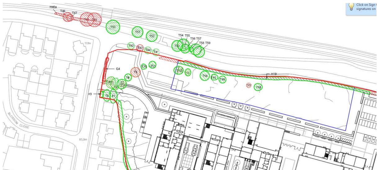
Image 9 – Plan showing main areas of tree loss with trees to be removed in red.
